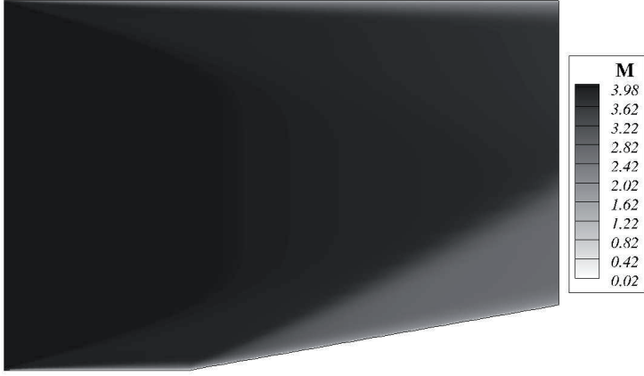
Figure 4.66: Mach number (M) contours in case of turbulent reacting flow in a ramped duct for T_{in} = 1200 [K].
