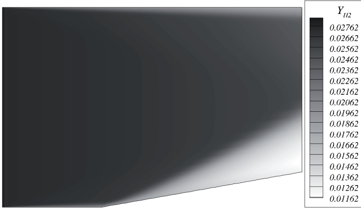
Figure 4.62: Mass fraction contours of Hydrogen ( Y_{H_2} ) in case of turbulent reacting flow in a ramped duct for T_{in} = 1200 [K].
