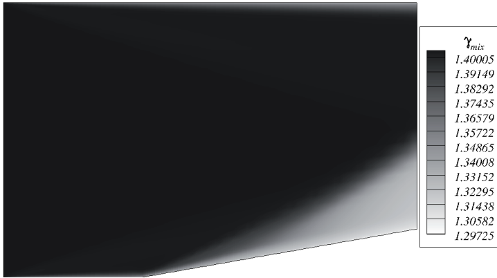
Figure 4.52: Mixture specific heat ratio ( \gamma_{mix} ) contours in case of turbulent reacting flow in a ramped duct for T_{in} = 900 [K].
