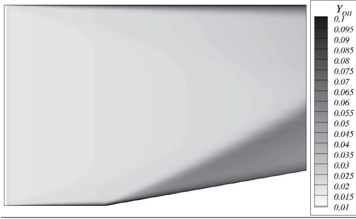
Figure 4.64: Mass fraction contours of Hydroxyl ( Y_{OH} ) in case of turbulent reacting flow in a ramped duct for T_{in} = 1200 [K].
