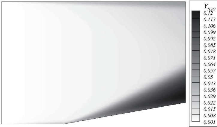
Figure 4.65: Mass fraction contours of water ( Y_{H_2O} ) in case of turbulent reacting flow in a ramped duct for T_{in} = 1200 [K].
