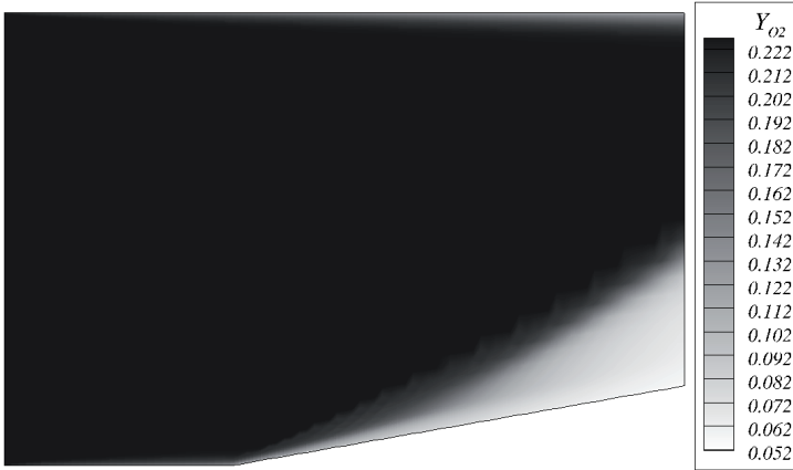
Figure 4.48: Mass fraction contours of Oxygen ( Y_{O_2} ) in case of turbulent reacting flow in a ramped duct for T_{in} = 900 [K].
