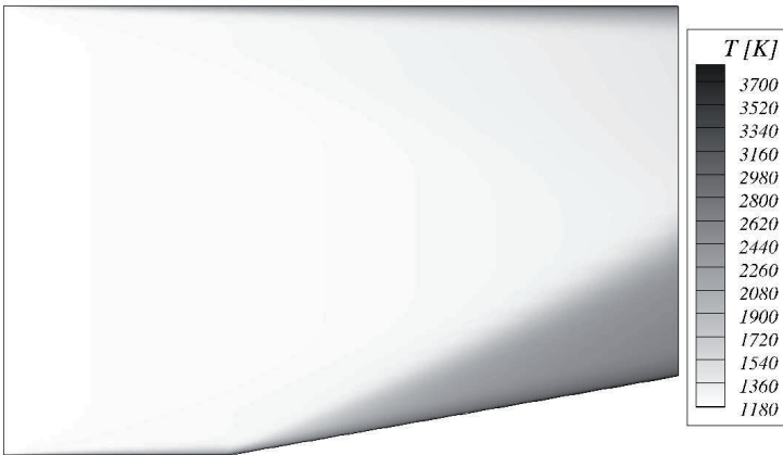
Figure 4.69: Temperature ( T ) contours in case of turbulent reacting flow in a ramped duct for T_{in} = 1200 [K].
