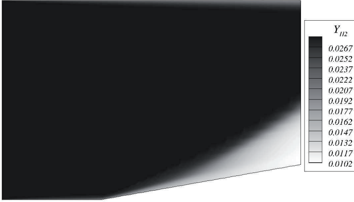
Figure 4.47: Mass fraction contours of Hydrogen ( Y_{H_2} ) in case of turbulent reacting flow in a ramped duct for T_{in} = 900 [K].
