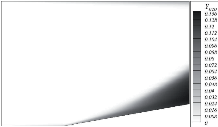
Figure 4.50: Mass fraction contours of water ( Y_{H_2O} ) in case of turbulent reacting flow in a ramped duct for T_{in} = 900 [K].
