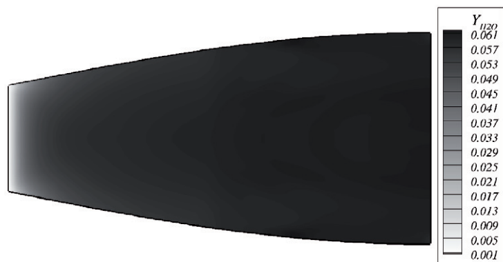
Figure 4.33: Mass fraction contours of water ( Y_{H_2O} ) for over-expansion through axisymmetric nozzle
