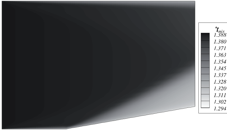
Figure 4.67: Mixture specific heat ratio ( \gamma_{mix} ) contours in case of turbulent reacting flow in a ramped duct for T_{in} = 1200 [K].
