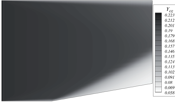
Figure 4.63: Mass fraction contours of Oxygen ( Y_{O_2} ) in case of turbulent reacting flow in a ramped duct for T_{in} = 1200 [K].
