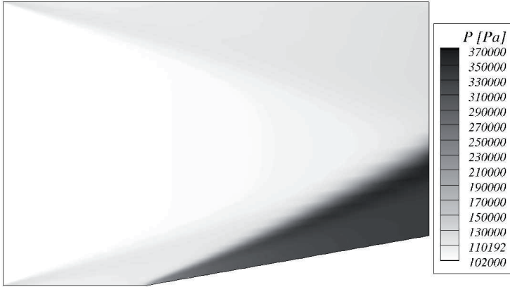
Figure 4.68: Pressure ( P ) contours in case of turbulent reacting flow in a ramped duct for T_{in} = 1200 [K].
