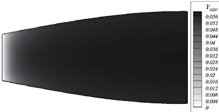
Figure 4.15: Mass fraction contours of water ( Y_{H_2O} ) for complete expansion through axisymmetric nozzle
