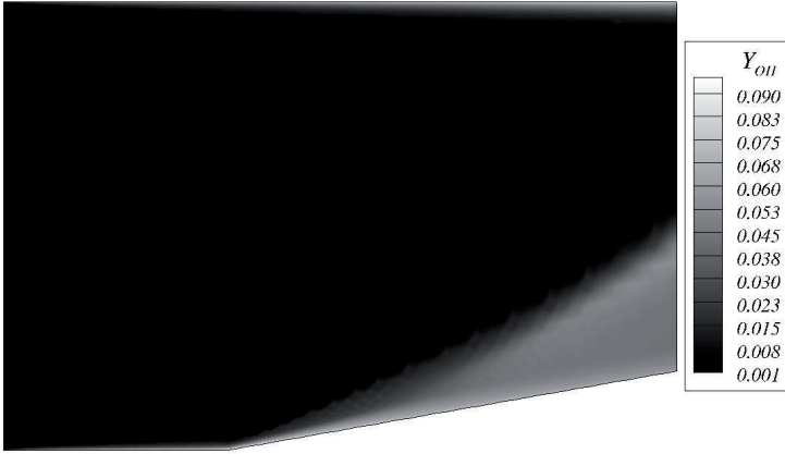
Figure 4.49: Mass fraction contours of Hydroxyl ( Y_{OH} ) in case of turbulent reacting flow in a ramped duct for T_{in} = 900 [K].
